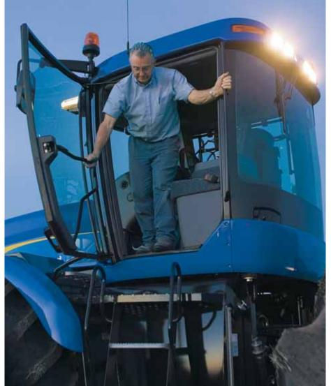
Convenient egress lighting lets you safely exit the cab while in a dark environment. Egress lighting is standard equipment on all T9000 models.
